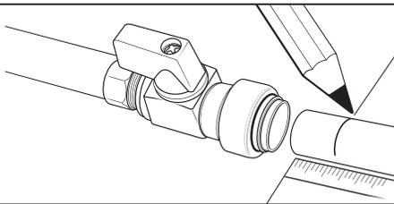
mark pipe exterior at 1" depth required for proper fit
