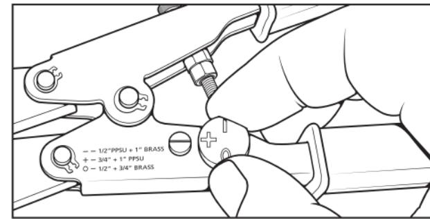
The PEX Ring Removal Tool is designed for use on all PEX rings.
